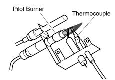
Figure 25 - Correct Pilot Flame Pattern
